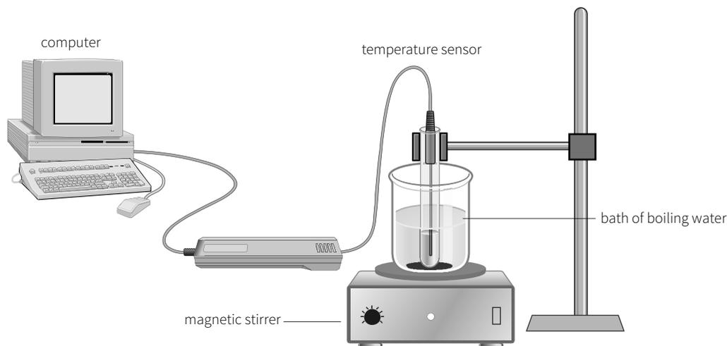
The temperature change was followed as the liquid was allowed to cool down. The data shown in Table 2.02 are taken from the computer record of the temperature change as the liquid cooled down to room temperature.
